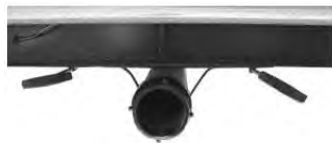
Black/Grey tank drain & valves
